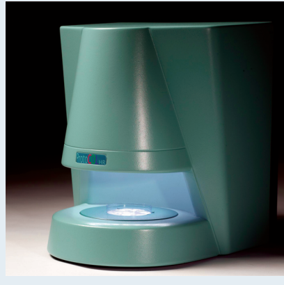
Photo 2: ProtoCOL system for automated post-OPKA colony counting
